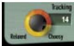
In order to accurately identify the pitch of the input, Auto-Tune 3 requires a periodically repeating waveform, characteristic of a voice or solo instrument. The Tracking control determines how much variation is allowed in the incoming waveform for Auto-Tune 3 to still consider it periodic.
