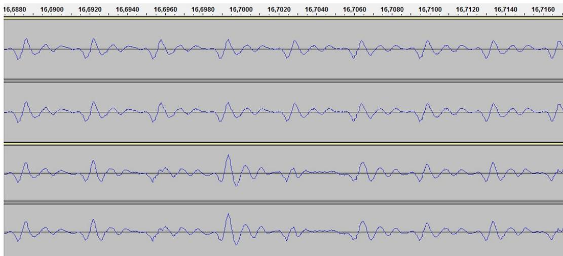
*Dry signal on top, processed signal on bottom (both are stereo). On steady state, latency is virtually zero.*
