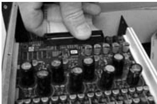
Pressing the 50-pin cable connector into the card
