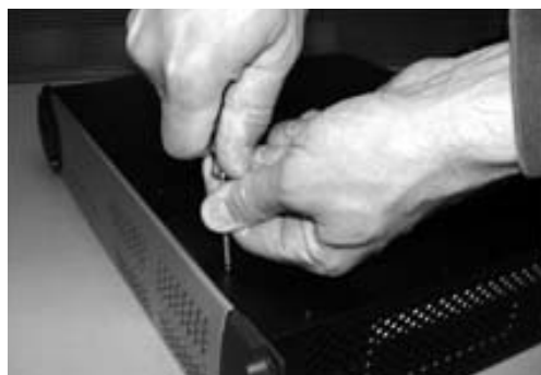
Removing the top cover screws
