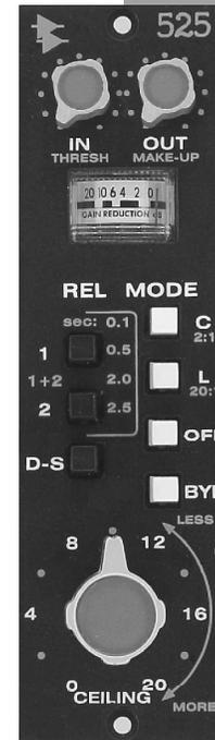
The API 525 is perhaps the most successful solid state feedback compressor in history. It delivers dynamics control behavior unlike VCA "feed forward" compressors so common today. A remarkable multi-function "ceiling" control can increase gain reduction (lower threshold) while simultaneously raising output level to match, so the user can alter dynamics "on the fly" without level changes.
