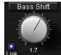
The Bass Shift is an „intelligent“ EQ band for the bass frequencies of your mix. We call it Bass Shift because 2 different frequencies will be „shifted“ against each other with the turn of just one knob. The frequencies have been pre-set and cannot be changed. If you are looking for a sweepable Bass- (and Presence-) Shifter please check out bx\_hybrid (available individually).
