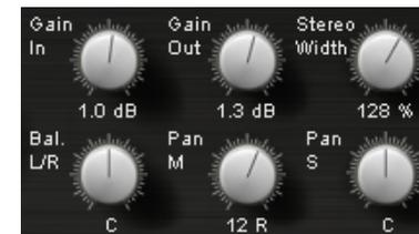
6 knobs to control general settings, independent of which mode is being used.
