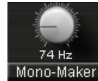
The Mono Maker will mono out the bass frequencies of your stereo mix, adjustable from 20 Hz up to 22 kHz, using M/S-technique even when the bx runs in L/R-mode.
