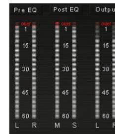
We have included dedicated LEDs for the Input Section (L&R), the M&S Section and the Output stage (L&R again), so you have total optical control over what you hear and what you do. Like with every other digital audio tool you should not push your levels into the red!
