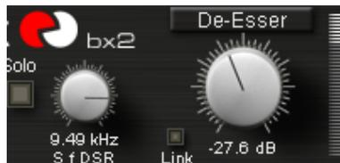
The bx\_digital De-Esser works with dynamic EQs that you can adjust to the needs of your mix. With the Solo buttons of the De-Esser section it is possible to listen to only the frequencies that you want to filter out of your mix.
