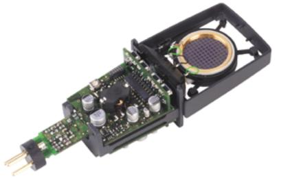
controlled in finer steps than on the microphone itself. You'll have access to 13 different polar patterns, 3dB steps for pre-attenuation and more. Controller commands to the microphone are sent over standard 3-wire XLR mic cables in short, coded tone bursts at supersonic frequencies.
